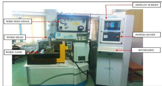
Figure 2.1: Pictorial view of WEDM machine tool
