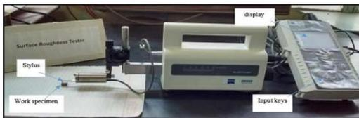
**Figure 2.2: photographic view of Surface Profilometer**
